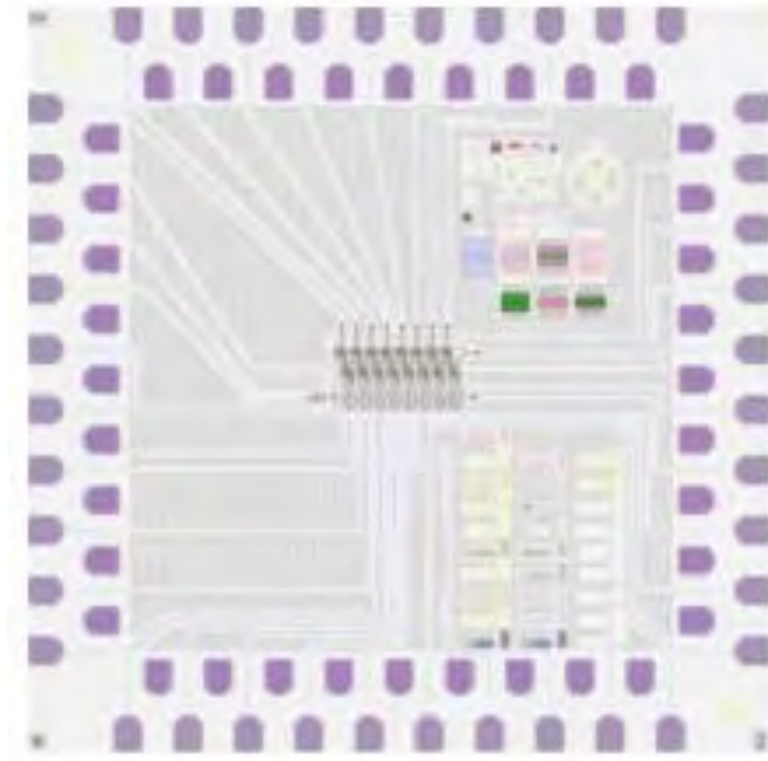
Fig. 2.1.4. The 8-bit RC adder on a 5x5-mm chip designed for HYPRES's 0.25- \mu\text{m} 4-layer process
