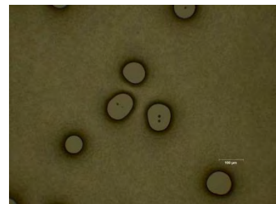
Figure 51 - Dewetting, high magnification
