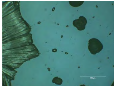
Figure 54 - High temp dewetting, crystallization boundary
