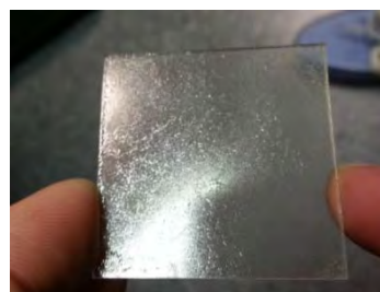
Figure 66 - Serpentine LC spray coating. Boundary not visible. Obvious disruption of film.
