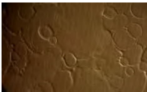
Figure 91 - Surface profile of the AZB coating on hard-coated PC plaque.
