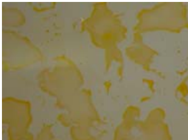
Figure 6 - Flame treatment, glass, 56x
