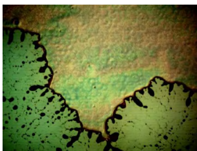
Figure 68 - LC spray coated onto AZB spray coated HCPC, boundary region.
