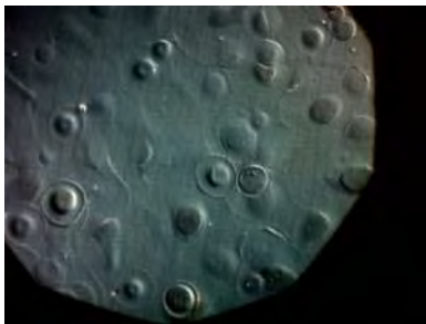
Figure 21 - AZB poor coating with rough surface
