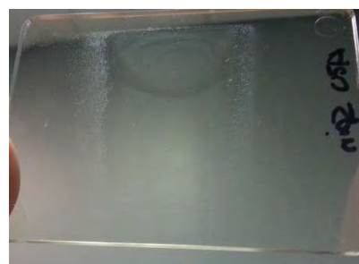
Figure 64 - Macroscopic view of LC spray coat pattern on HCPC. Boundary area observable. Pooling of coating observable at start position.
