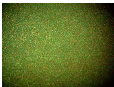
Figure 67 - LC spray coated onto AZB spray coated HCPC, center region.
