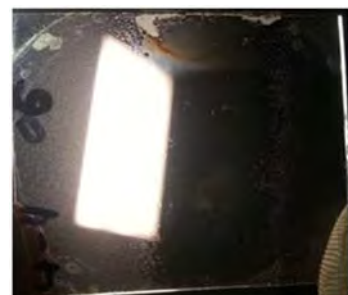
Figure 61 - Macroscopic view of spray coat pattern on glass. Transparent area was irradiated. Boundary area observable.
