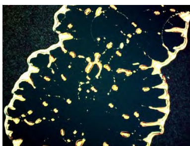
Figure 71 - Local dewetting of spray coated LC on spray coated AZB HCPC.
