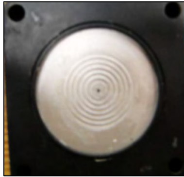
Figure 17. Fabricated bull's-eye structure with six periodic grooves covered with the silver film.
