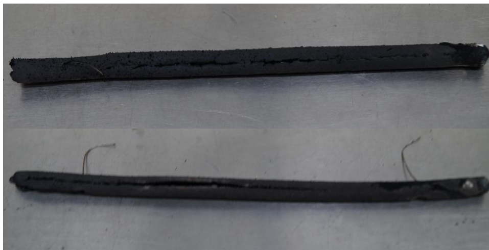
Figure 5: Burned strands showing splits in the coating – 4.09 MPa (top) and 8.01 MPa
