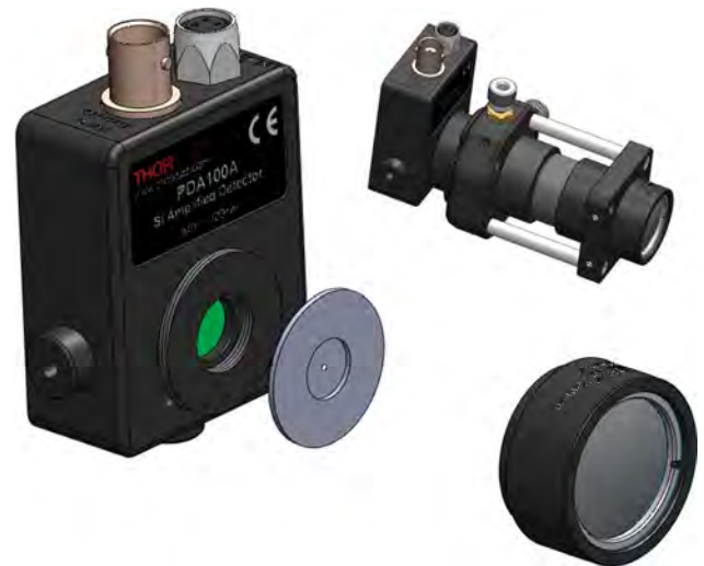
Fig. 6. Computer aided design drawing of the NAAD showing the lens (right), aperture (middle), and detector surface (left). The inset shows a drawing of the fully assembled NAAD.
