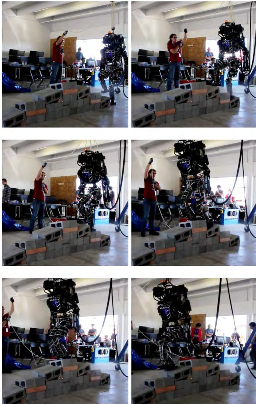
Figure 4.8: Snapshots of the Atlas robot walking up and then walking down the tilted cinder blocks.
