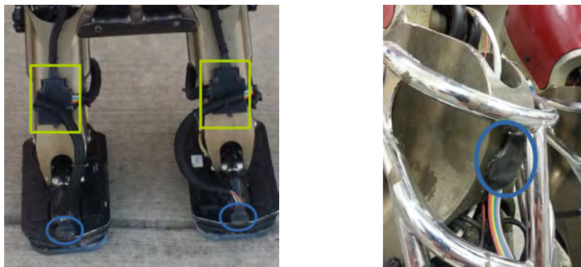
(a) Feet IMUs in the blue circle, sensor nodes in green box (b) Shin IMUs right below the knee in the blue circle
