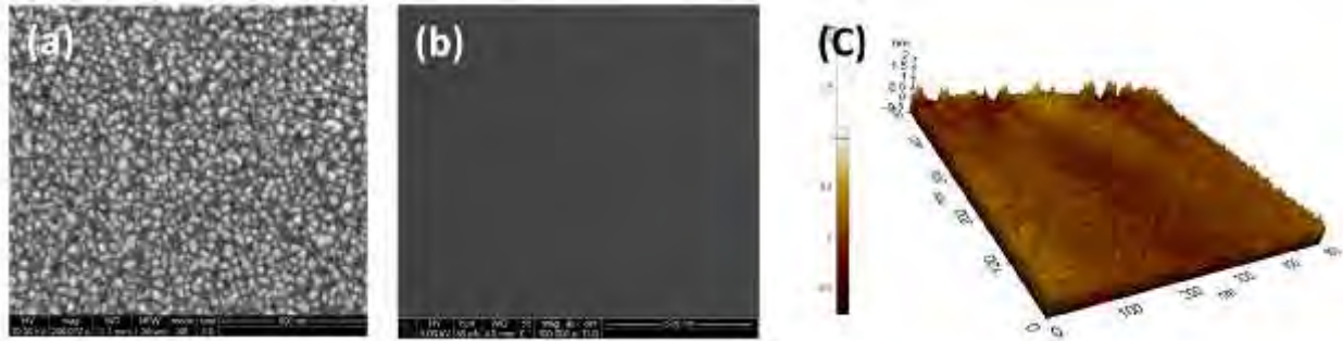
Fig. 3 Scanning electron microscope image of surface of silver film grown (a) without a wetting layer and (b) with a wetting layer of Ge. (c) Atomic Force Microscope image showing ultra-smooth surface topography of the film grown using the wetting layer.
