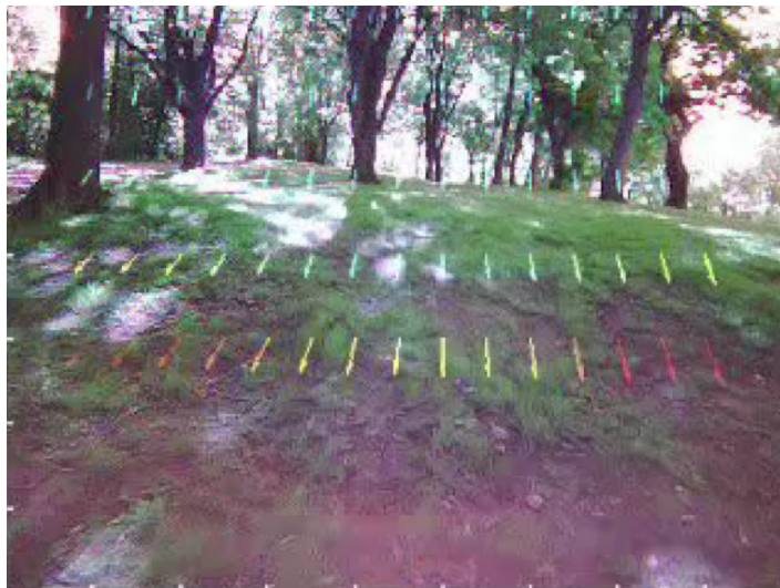
(d) Temporal information is maintained by computing optical flow statistics over the image, statistics of which are then used as features in the learning algorithm for depth prediction.
