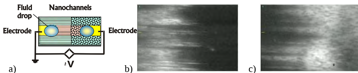
Figure 6. (a) Sample with nanochannels on the left and porous media on the right, (b) DNA accumulation on media separation, (c) DNA penetration in porous
