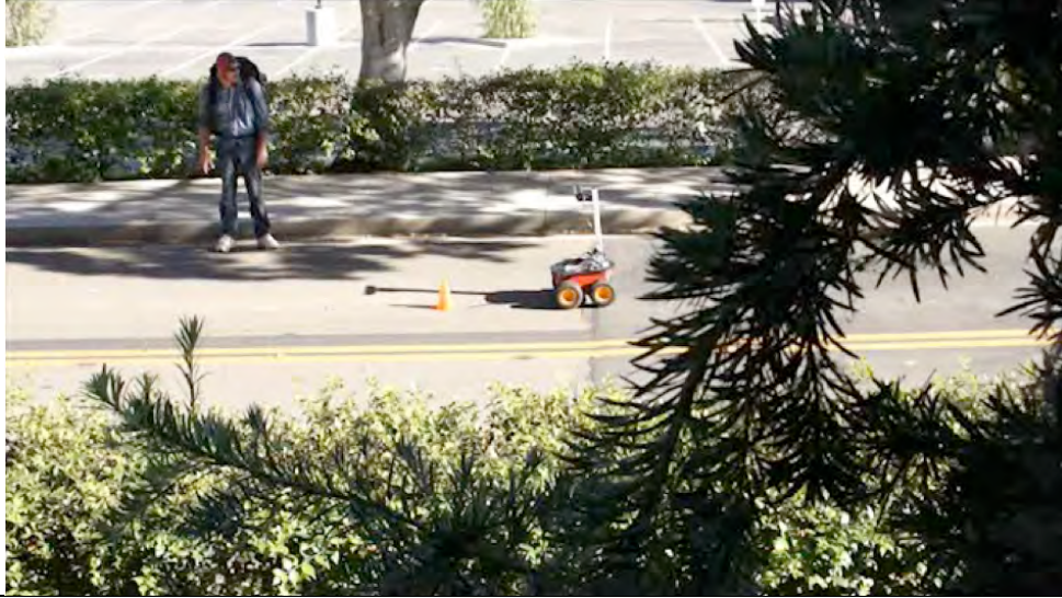
Figure 16. Mobile subject Hagedorn with red EEG gel cap controls navigation of robot (center). A signal-processing computer within the backpack worn by the subject communicates wirelessly with a computer onboard the robot. EEG signals are processed by the computer in the backpack to control the robot's left/right turns and starting/stopping. Subject's task is to cause the robot to navigate a full lap of a slalom course marked by orange pylons.
