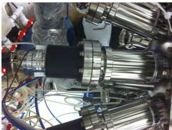
Figure 22. Photograph of the installed oxygen resistant Zn source on the MBE growth system.
