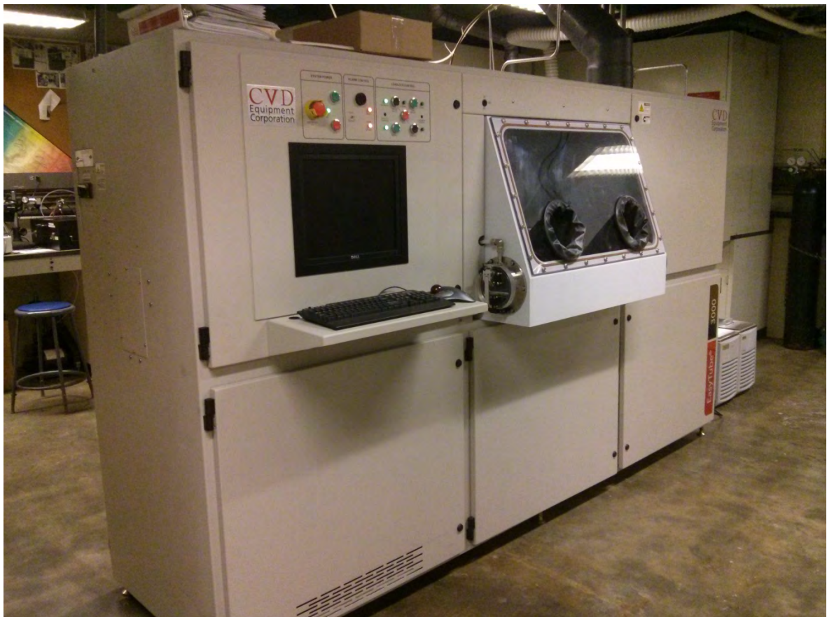
Figure 1 Photo of MOCVD reactor installed at RPI Johnson Engineering Center room 7218 during Spring of 2013.
