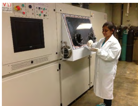
Figure 3 A wafer of p-GaAs is being loaded to the system for growing ZnTe. The wafer is being used to fabricate single crystal CdTe solar cells (funded by First Solar)
