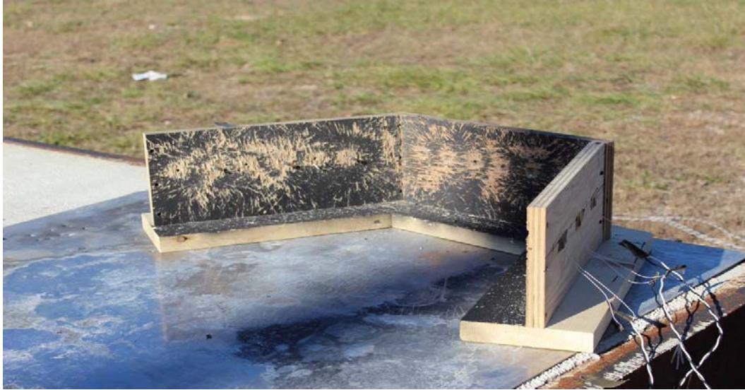
Fig. 2 Fixture used for detonator-only experiments
