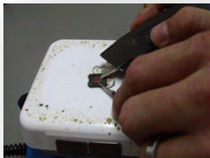
Counterfeiter removing die from part
