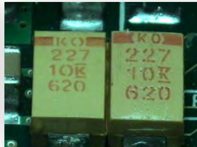
Marking slightly different on counterfeit part
