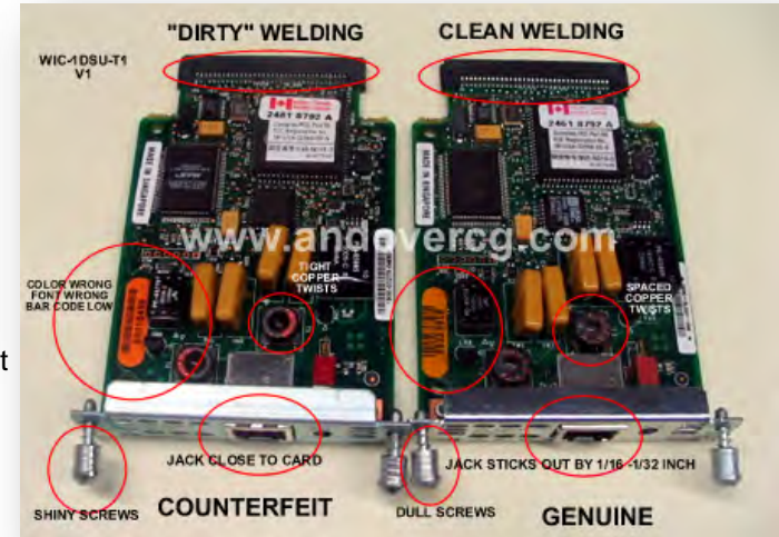
Marking slightly different on counterfeit part
