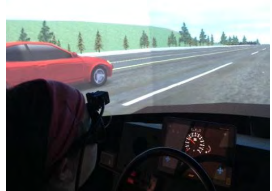
Figure 9. Driver wearing eye tracking glasses while performing the Operational Peripheral Vision Test
