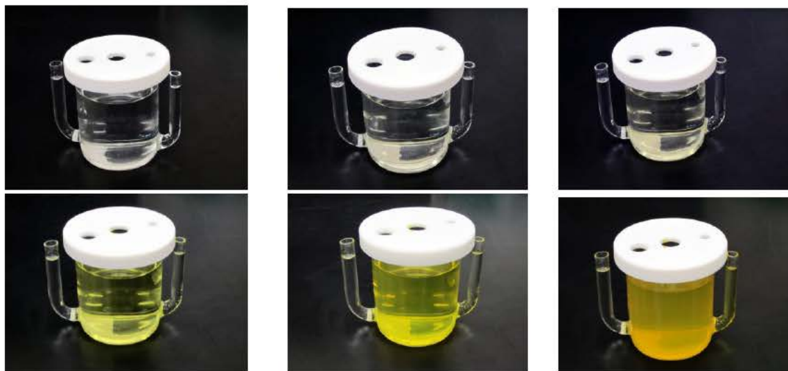
Fig. 6. Images of 0.01 M acetaldehyde + 1 M NaOH solution (a) before acetaldehyde added; (b) 2 min, (c) 10 min, (d) 0.5 h, (e) 1 h, and (f) 2h after acetaldehyde added.
