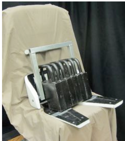
Final installation with back angle measurement tool
