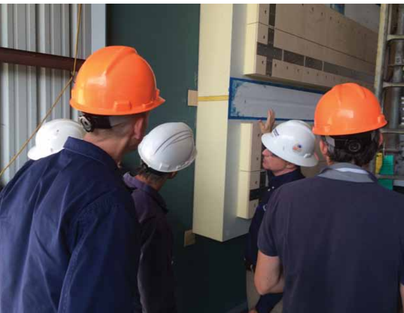
Liquefied Gas Carrier NCOE personnel examine a cargo containment system mock-up. U.S. Coast Guard photo.
