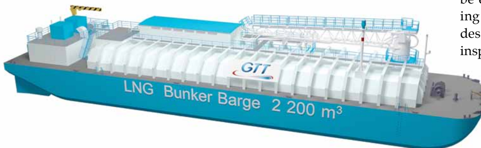
An example of an LNG bunker barge. Image courtesy of GTT North America.
