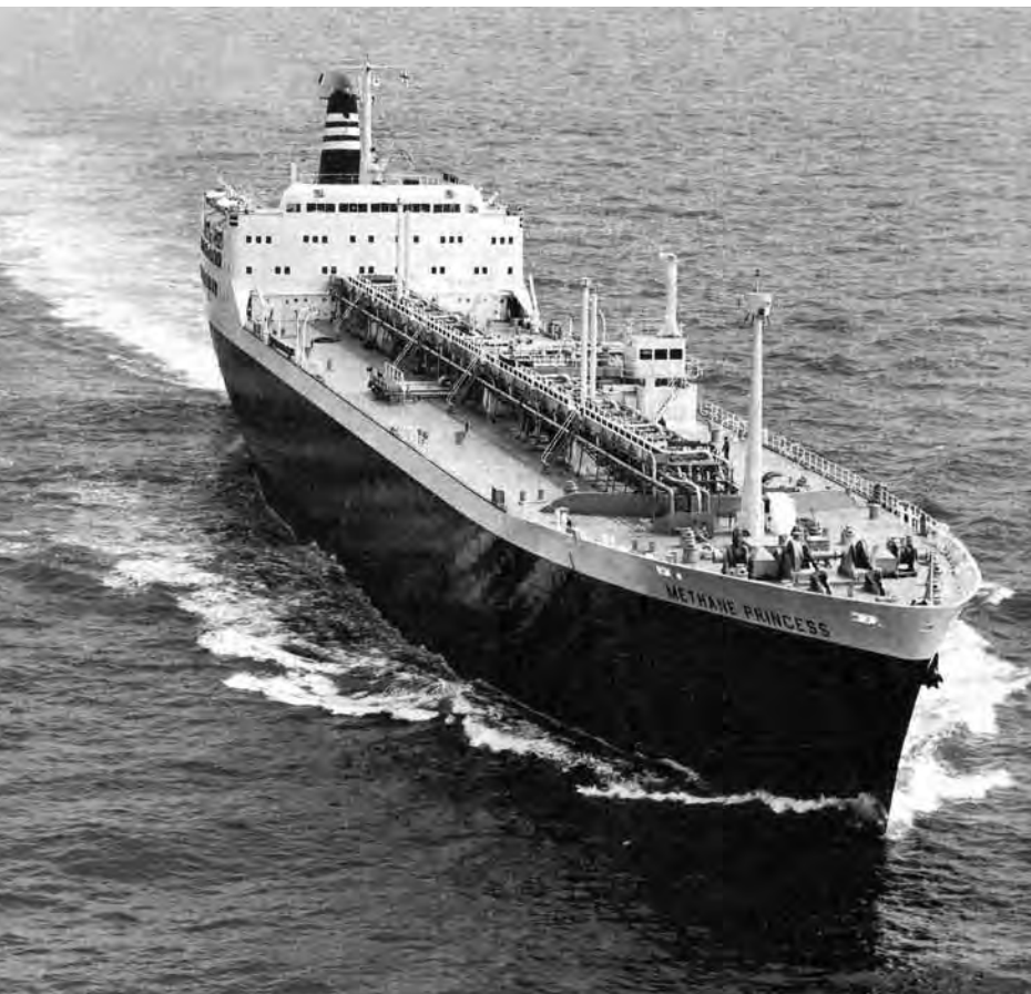
The Methane Princess is the first commercial LNG vessel; she entered service in 1964. Photos courtesy of the Society of International Gas Tanker and Terminal Operators Ltd. (SIGTTO).
