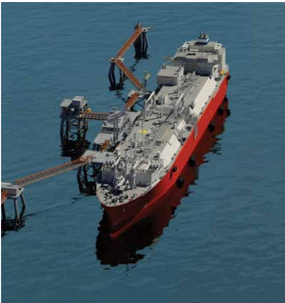
An FSRU gas port.
