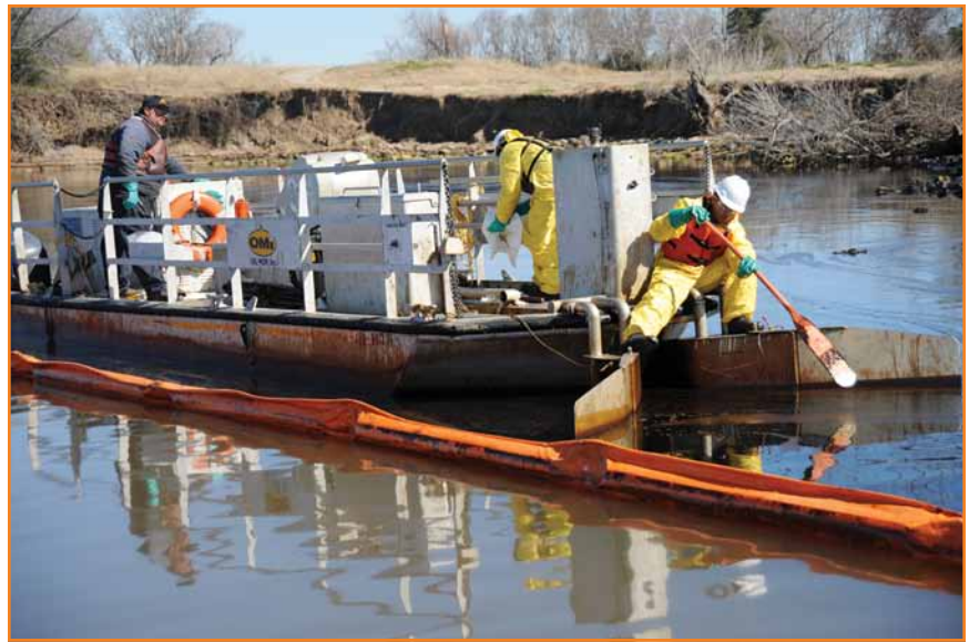
Oil spill response team members force oily water into a skimmer. U.S. Coast Guard photo by Petty Officer Tom Atkeson.
