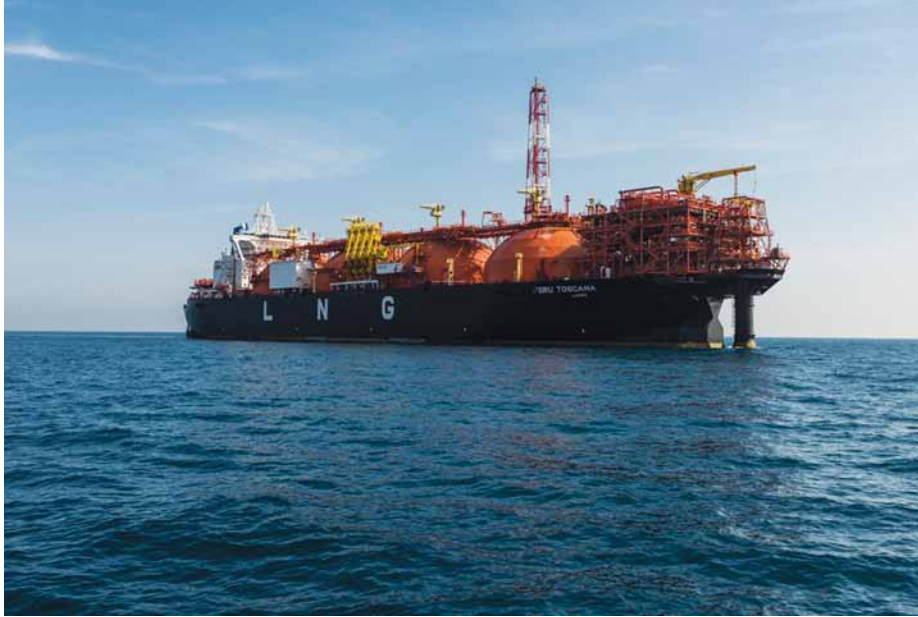
The floating storage and regasification unit is essential LNG infrastructure.
