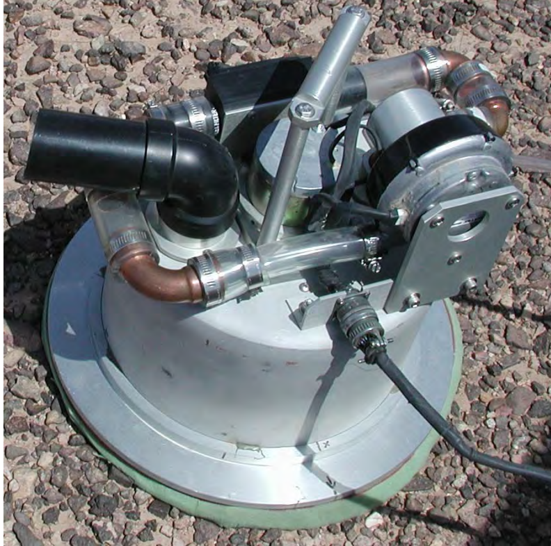
Figure 5. The PI-SWERL ® instrument on a test surface for measuring PM 10 dust emission potential in situ.
