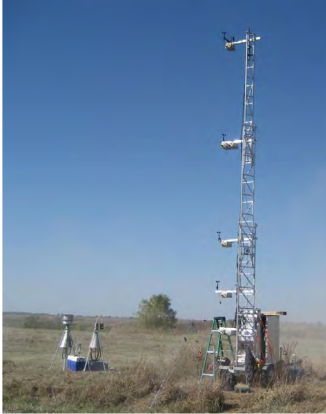
Figure 2. Flux tower (right side of frame) and medium volume PM 10 and PM 2.5 samplers deployed to measure dust plumes characteristics generated by vehicles traveling on an unpaved road.
