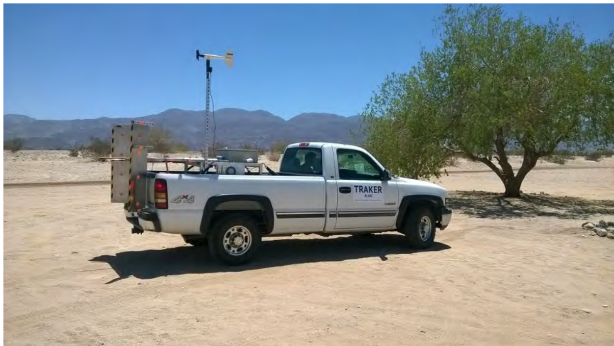
Figure 3. TRAKER™ III. Instrumentation is held within the bed of a standard pickup truck and dust concentrations created by vehicle travel are measured in the lee of the custom-designed baffle mounted to the truck's rear bumper.
