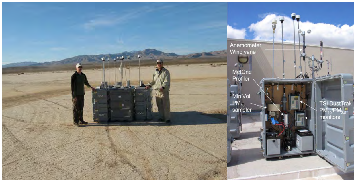
Figure 7. The four dust deposition instrument enclosures set up for the initial collocated precision measurements (left panel) and the instrumentation inside (right panel). Note the anemometer and wind vane are not at the height used during field measurements, which matched the height of the PM inlets.
