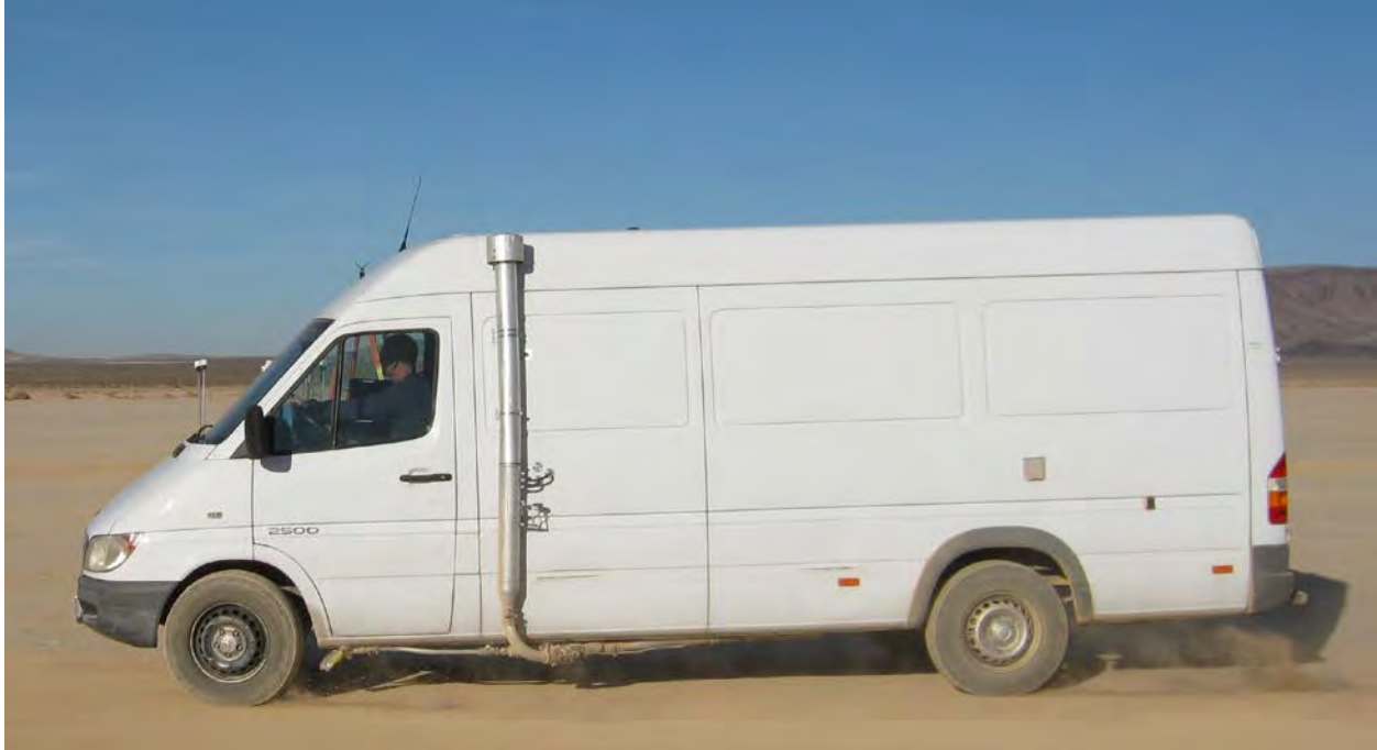
Figure 4. TRAKER™ II. Instrumentation is within the van and dust concentrations resulting from vehicle travel are measured behind both front tires.
