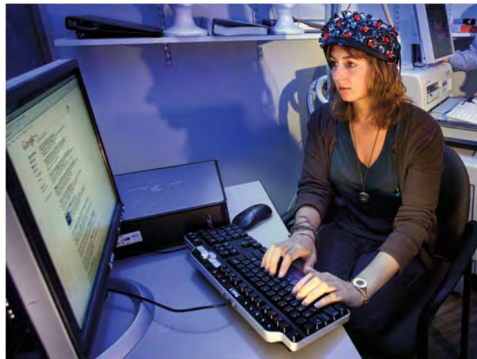
Figure 1: The ETG4000 52-channel fNIRS at Newhouse.
