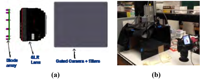
Figure 4: Novel Dynamic optical Contrast Imaging (DOCI). (a) CAD design of large FOV system. (b) Assembled system used in ex vivo imaging study.
