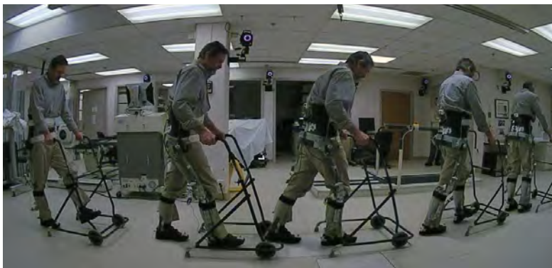
Figure 21. Subject walking with instrumented brace with embedded controller collecting and transmitting data to PC.
