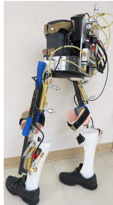
Figure 17. Assembled exoskeleton for HNP2.
