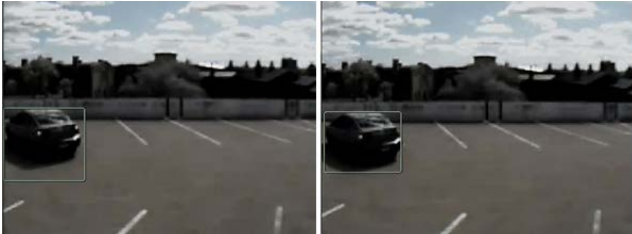
Figure 5. Same Vehicle Tracked Using the RGB Background Model (Left) and Ciel*A*B* Background Model (Right) Results in a Tighter Object Bounding Box Reducing the Effects of Changes in Scene Illumination
