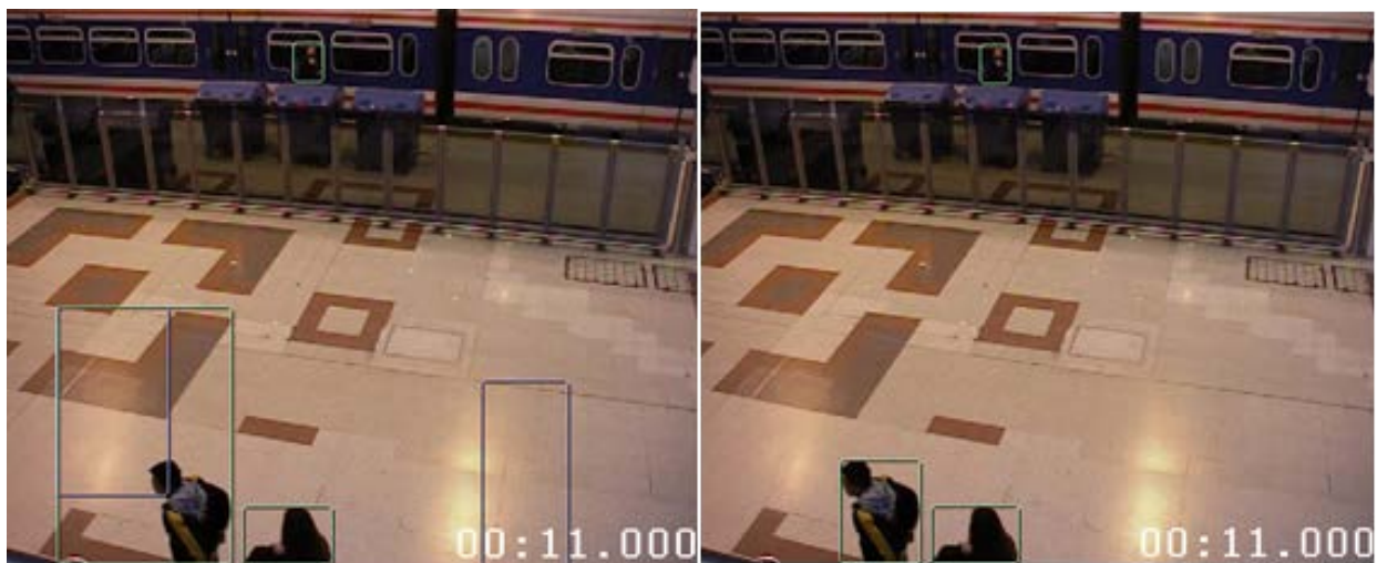
Figure 10. Factors Such as Lighting Changes May Cause These ‘Ghost’ Objects to Linger and Detected as Idling (Left), the Updated Object Removal Algorithm Reliably Removed These Spurious Detections (Right)
