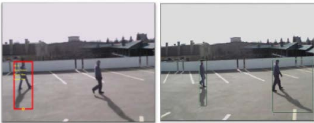
Figure 6. Example of Missed Detection by Primordial [Using IntuVision SDK] (left) And Detection of the Same Object by IntuVision Processing (right) Using Same Settings
