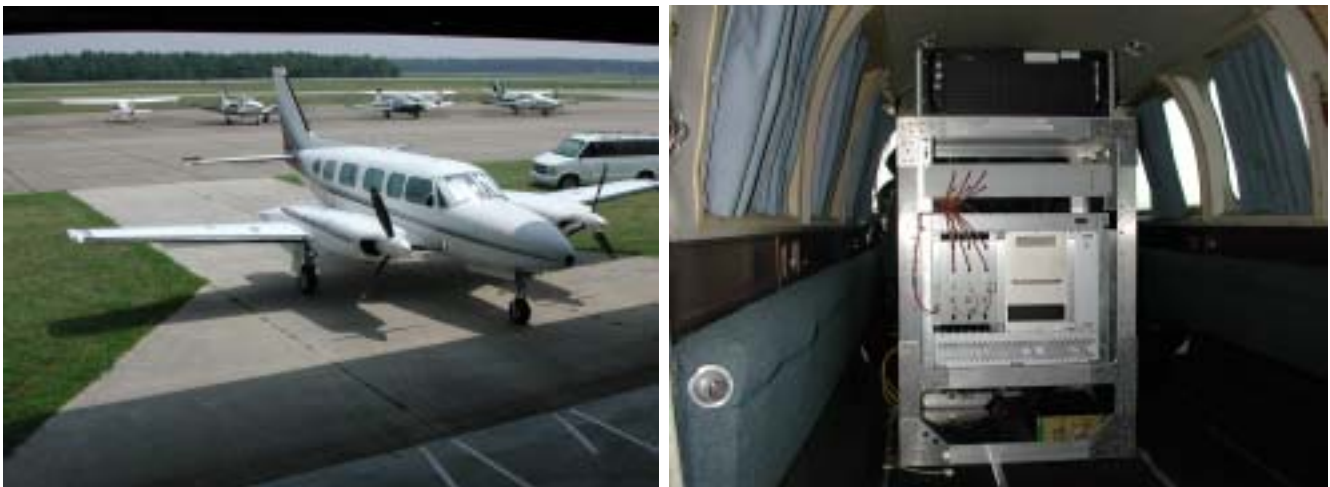
Figure 1. Johns Hopkins Applied Physics Laboratory surface reflection receiver installed in light aircraft for first experimental flight series.
