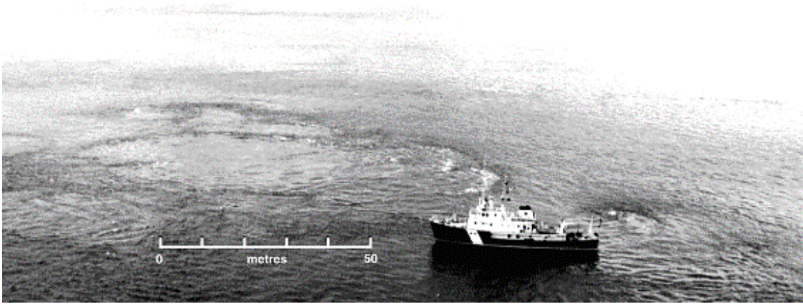
Figure 3a Aerial photograph showing the CGS VECTOR in a zone of intense turbulence and eddy intensification associated with the tilting of separated flow downstream of a headland.
