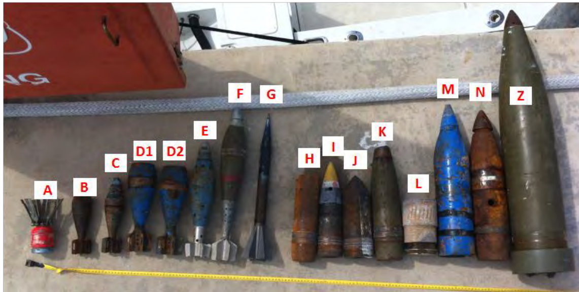
Figure 4. Test targets used for data collection near Key Biscayne: A - BDU-28 Submunition, B - 60mm Mortar (without fuze nose, pitted brown, with tail), C - 60mm Mortar (with fuze, with tail, inert training round; ATC standard target), D1 - 81mm M43A1/M49A2 Mortar (Blue Training Round, No Fuze), D2 - 81mm M43A1/M49A2 Mortar (Blue Training Round, No Fuze), E - 81mm Mortar (with fuze), F - 81mm M821A1/M889A1 (empty) High Explosives (HE) Mortar (with fuze), G - 2" Rocket APFSDS-T M735, H - 76mm Projectile (no fuze), I - 3" Armor Piercing Projectile MK28 Type A, J - 90mm Projectile (no widescreen), K - 90mm High Explosive (HE) Projectile M71, L - APDS Adapter with End Cap and Cartridge, M - 105mm Projectile (Blue Training Round), N - 105mm Projectile (with band and solid tip), Z - 155 mm Howitzer Projectile.
