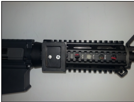
Figure 6. Custom plastic sensor mount. The accelerometer should fit snugly within the mount and the mount should be secured to the Picatinny Rail Mount so there is no noise that is not from the weapon being fired.
