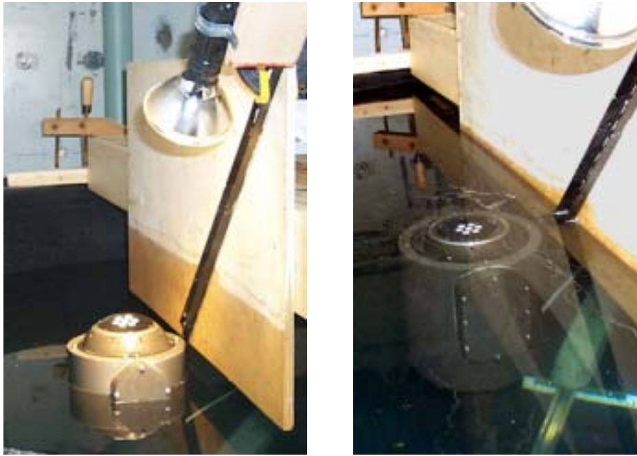
Figure 2. Pictures of the radiometer sensitivity test made in the SSI test tank. Measurements were made with the device below water level and a light source in air. The output of the 7-wavelength SATLANTIC radiometer was recorded as a function of in-air light incidence angle. Measurements were made with and without the glass dome of the ISPS covering the radiometer.
