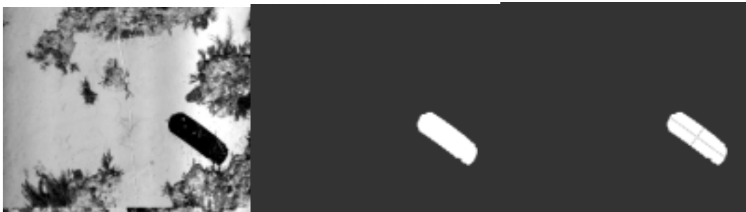
Figure 2 . Enhanced image (left), detected image (middle), and detected and segmented image (right) for a laser line scan image. The object length, width, area and orientation is computed at this point.
