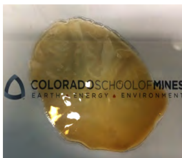
Figure 7. Image of a PPO-TPQP-40 film from drop casting from DMSO.
