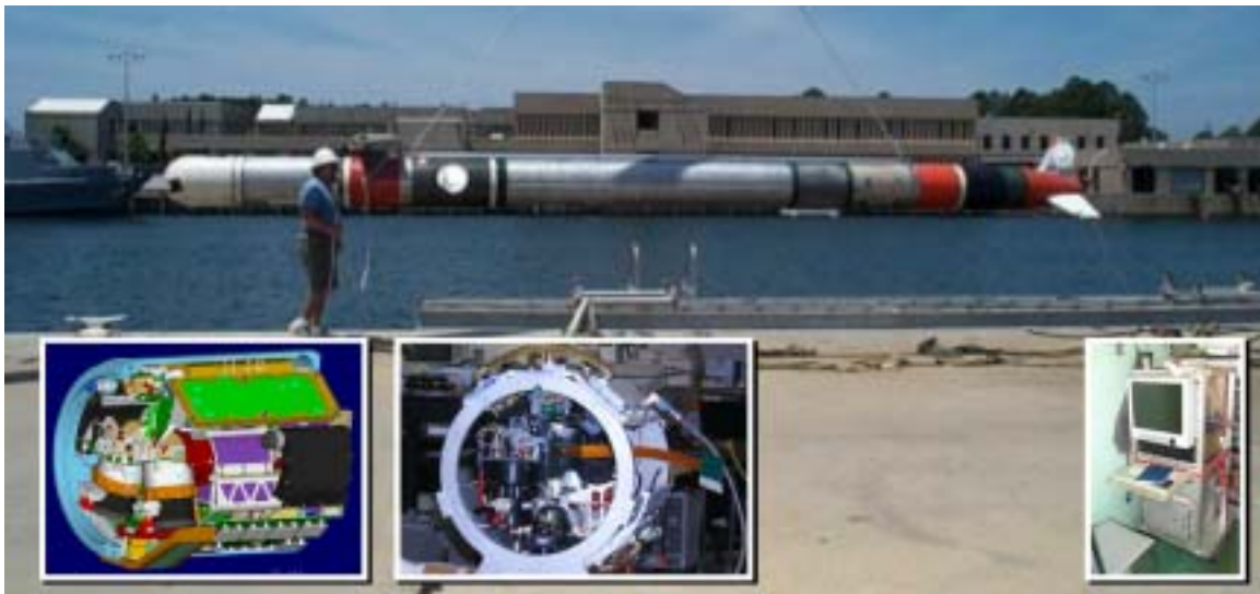
Figure 1: STIL, Processing System, and EOID Multi-sensor Tow Body [Tow body shown dockside with STIL sensor integrated in small section ahead of the tow body wing. STIL CAD drawing. STIL Sensor in Laboratory. Topside processing system as deployed onboard ship ]
