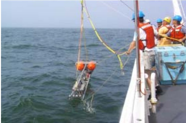
Figure 1. Deployment of the Optical/Acoustic Drifting Buoy off the R/V Endeavor near New Jersey Coast, July, 2001. The package contains optical, acoustic and chemical measurement systems designed to examine the influence of bubble clouds on upper ocean hyperspectral reflectance.
