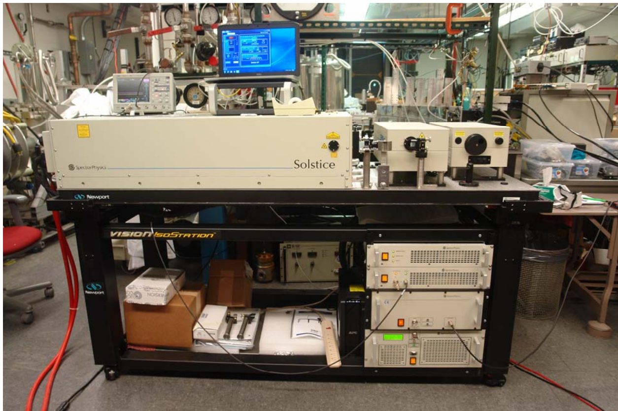
Figure 7. The laser system for Femtosecond Laser Electronic Excitation Tagging (FLEET)
