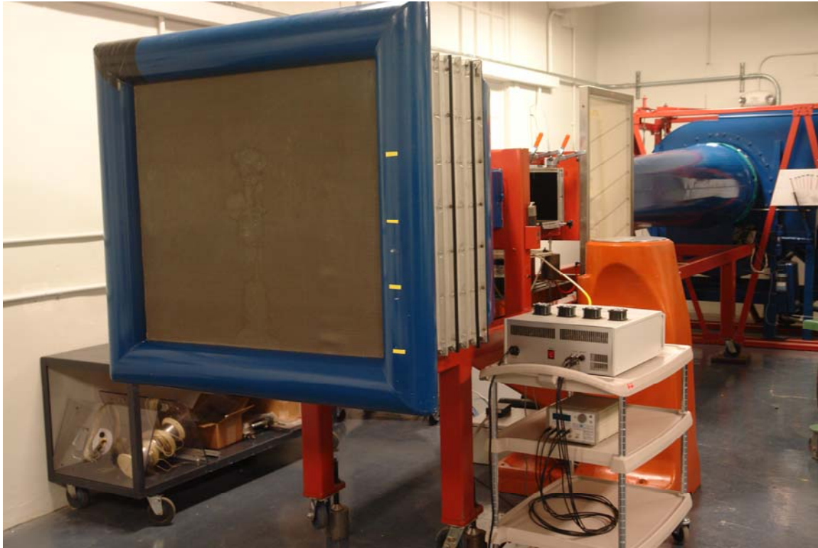
Figure 1. Subsonic Variable Speed Plasma (SVSP) blow-down wind tunnel.
