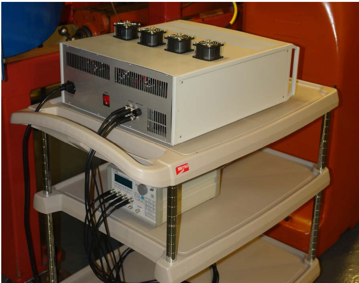
Figure 5. FID 4-channel pulser and BNC synchro-generator. The pulser operates in burst mode synchronized with the model pitching by NI interface.
