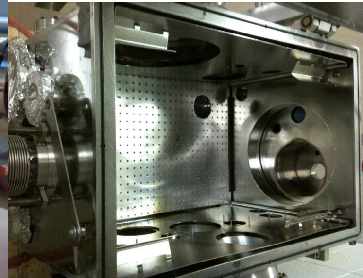
Vacuum Chamber 1x0.5x0.5 m 3
