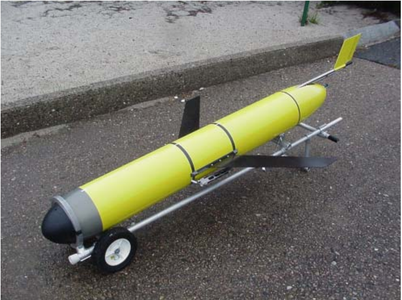
Figure 1: Redesigned Slocum electric glider. Major improvements include addition of a modular science payload bay (center section) with a dedicated computer system, integration of acoustic transducers in the bow cone for underwater communications, and addition of a servo-controlled rudder for improved lateral control.
