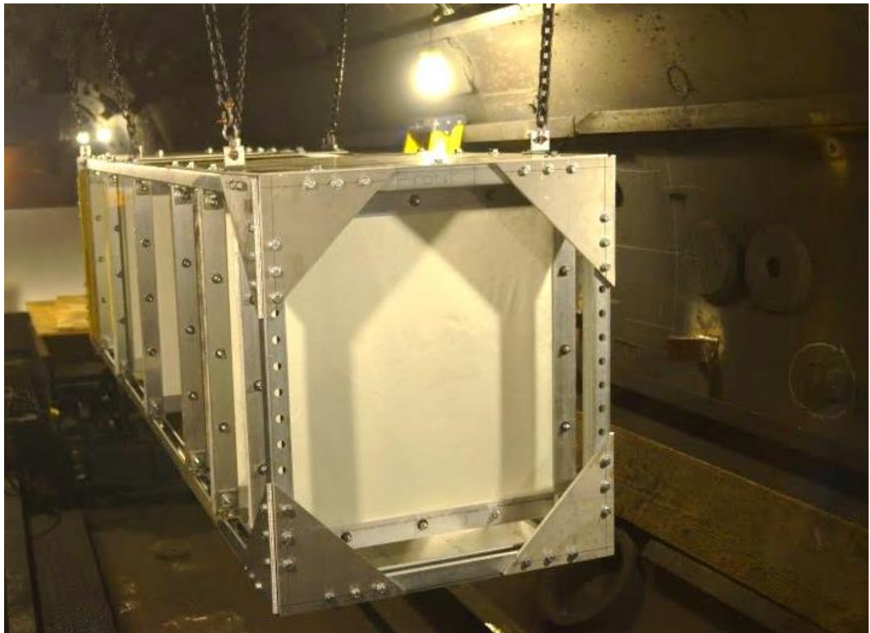
Figure 2. Shock Shield Installed in Range G Tank
