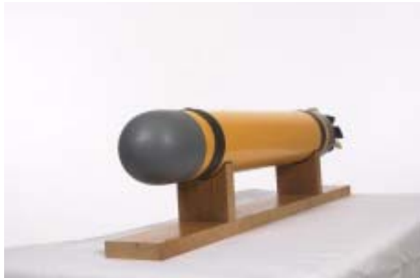
Figure 2. USNA-1, a micro autonomous underwater vehicle designed at the U. S. Naval Academy for experiments in controlling platoons of underwater vehicles.
