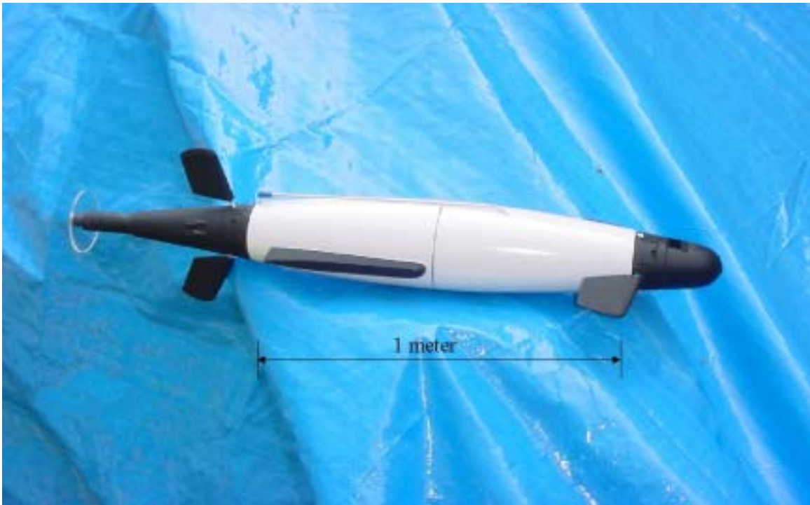
Figure 1. Small AUV to be Used as Test-bed Vehicle. [A small AUV, roughly 2 meters long, will be used to test the developed techniques.]
