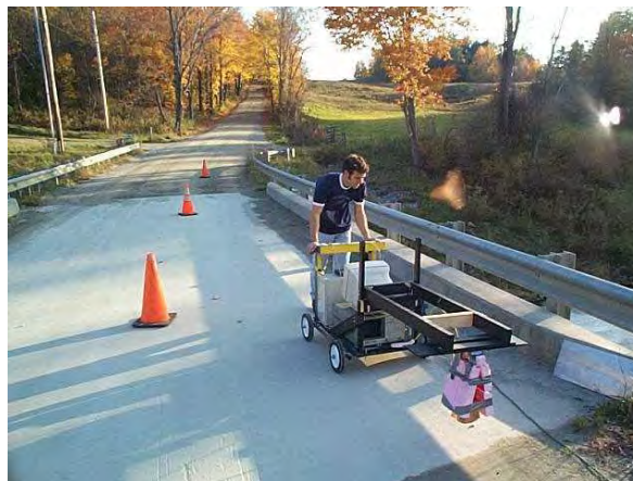
Figure 13 Use of linear vector network analyzer for penetrating radar scan of Turkey Lane Bridge deck (Hinesburg, VT, circa 2003)
