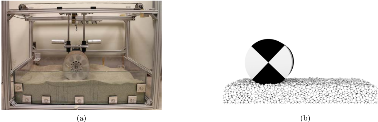
Figure 10: A photograph of the single wheel test experiment at MIT’s Robotic Mobility Group [19] (left), Chrono simulation of the single wheel test (right).
