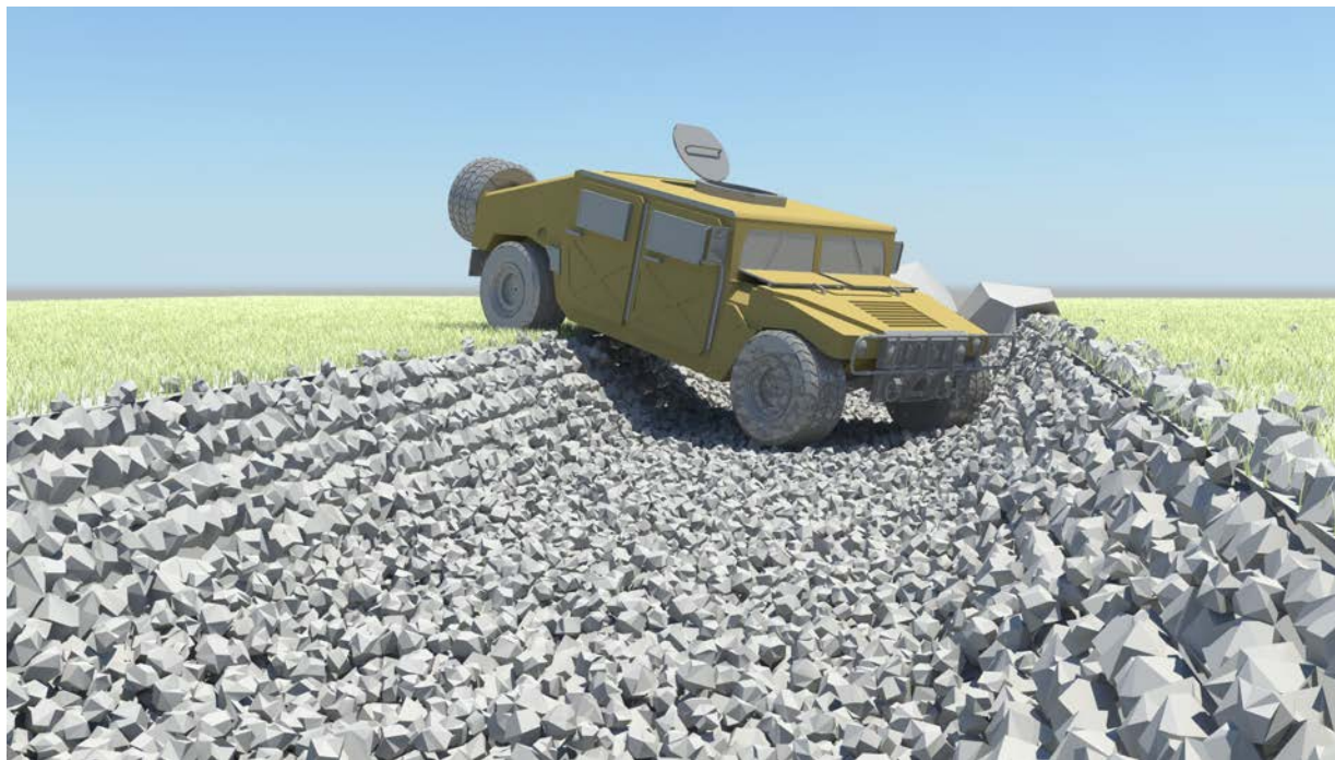
Figure 1: A HMMWV traversing a deformable terrain modeled using the discrete element method (DEM).
