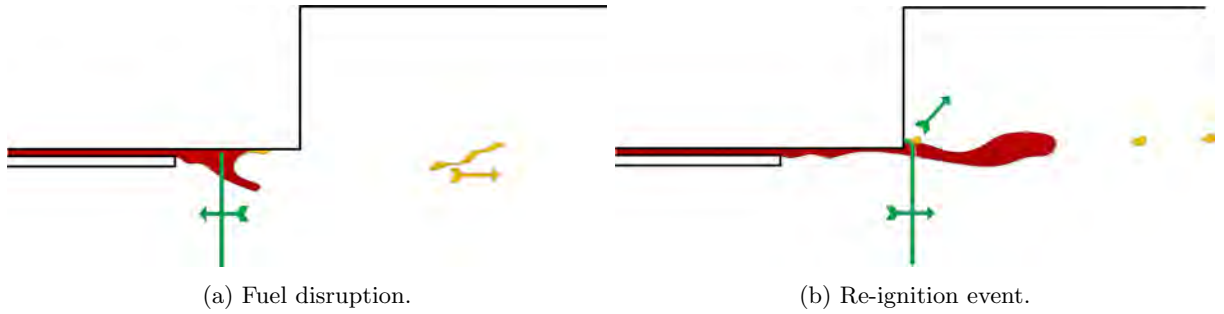
Figure 3: Key events in the CVRC instability mechanism. In both figures the red is unburnt fuel, the yellow is combustion and the green is the oxidizer pressure pulse. In (a) the oxidizer pressure pulse is moving from the combustor into the oxidizer post, when it passes by the fuel it creates a temporary stoppage in the supply. Increased mixing due to the baroclinic torque leads to combustion in the cup region. For the reignition shown in (b) the oxidizer pressure pulse travels from the oxidizer post into the combustor, in doing so it pushes unburnt fuel into the warm recirculating gases near the dump plane which leads to combustion and a rapid burning of the unburnt accumulated fuel.
