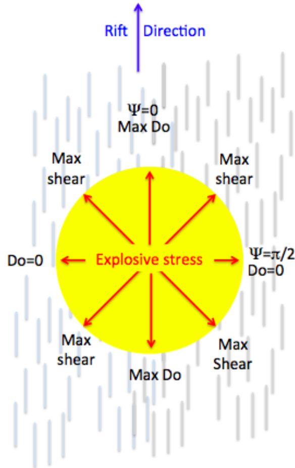
Figure 5. Explosion in granite that has a preferred fracture orientation (rift plane). In this case, the angle \Psi between the largest principal compressive stress (radial) and the rift plane varies as indicated.
