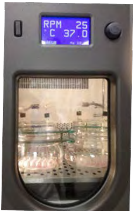
Figure 2. Two Custom-Made Glass Chambers with 24-Well Plates in the Incubator. One chamber is for the control exposure, and the other for the toluene exposure.
