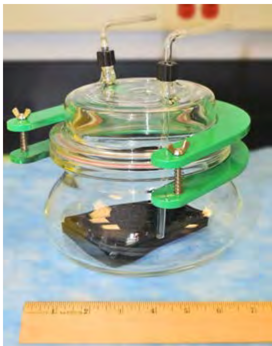
Figure 1. A Custom-Made Glass Chamber with a Lumox ® 24-Well Plate. Chamber dimensions are 7 inches wide by 6 inches high.
