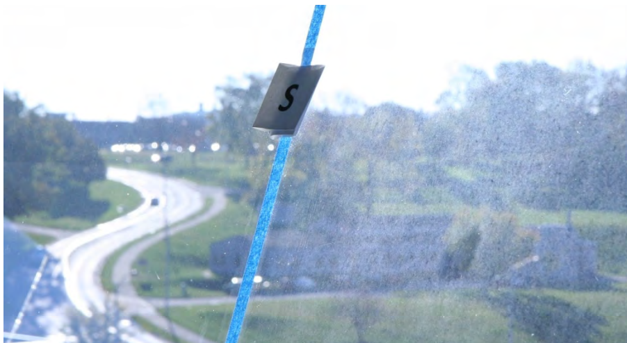
Figure 2. Contrast loss on coated side (right of blue tape) due to light scatter from setting sun.
