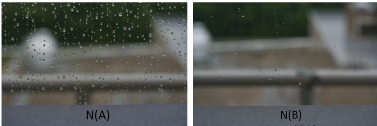
Figure 1. Effect of SNP coating on distribution of water droplets from rain (left is uncoated, right is coated).
