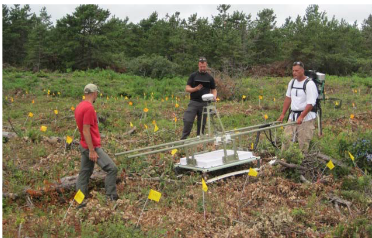
Figure 3-1 - TEMTADS 2x2 sensor in litter-carry mode configuration at MMR in 2013
