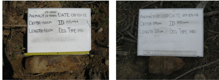
Figure 9-3. Examples of the partial shells successfully classified at TOI in this demonstration
