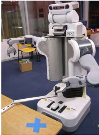
Figure 13: PR2 robot manipulating an crank (described by a revolute model)
