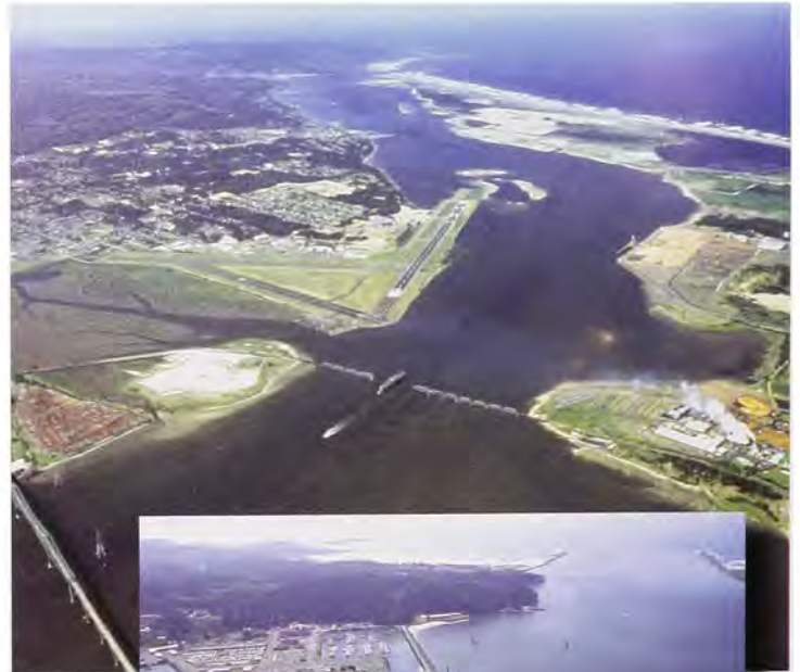
The extended training jetty joined with the south jetty at Umpqua River. Dredging at Coos Bay to deepen the Coos-Millicoma channel for deeper draft ships allowing the Port to stay competitive.
