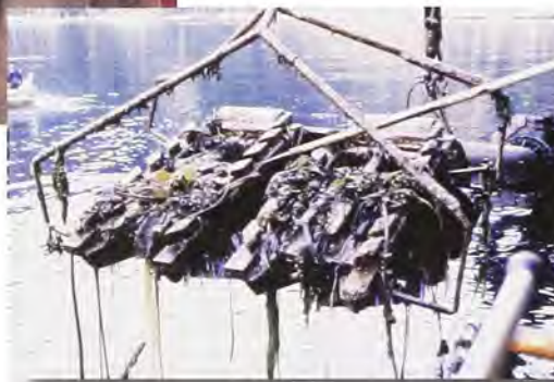
Motor launch pushed the oil boom close to the dredge for oil removal. The cage system for the drag head helped keep large debris away from the suction head. Oil in the hold of the dredge was taken to the dock for transfer to awaiting trucks.
