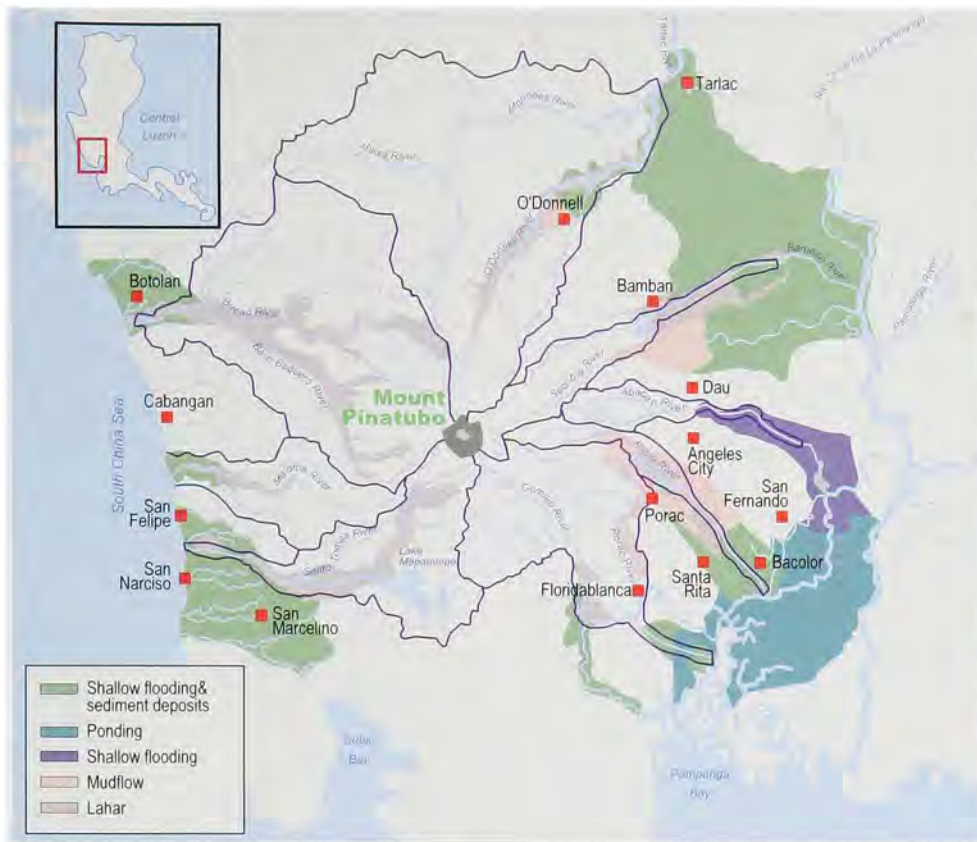
Mt. Pinatubo devastation area map and Corps of Engineers recovery plans for sediment retention, channel excavation, and levees
