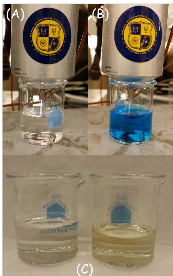
Figure 1. (A) AC jet in direct contact with Au electroless solution, (B) Ni electroless solution, and (C) Sn electroless solution after plasma exposure showing minor color change from clear to light brown-right hand side.
