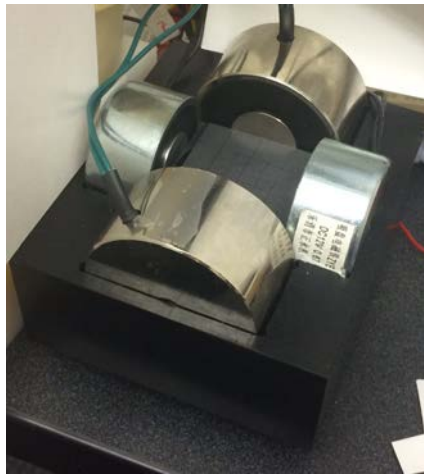
Figure 3.9: Our final magnetic setup includes 5 magnets. Two pairs to achieve a uniform field in the x,y axis and z magnet (not shown) pointing up.
