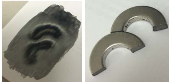
Figure 3.6: A spatially varying magnetic field can be used to create spatially varying reflectance. A coating of nail polish was applied on paper while the two magnets on the right were place 3mm below the paper. The resulting flake orientations gives the impression of a bump map. We remind the reader that this print is completely flat.
